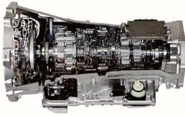
Fig. 3 Front-Engine Rear-Wheel Drive 10-Speed AT for the Toyota Land Cruiser 300
