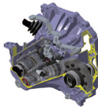
Fig. 1 Appearance of Daihatsu Front-Engine Front-Wheel Drive 5-Speed MT
