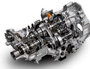
Fig. 8 Cut Model of Daihatsu FR-CVT
