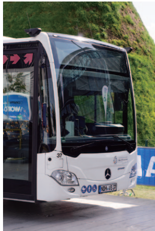
Fig. 31 Optical Mirror System Replacing Side Mirrors
