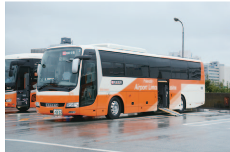
Fig. 14 Mitsubishi Fuso Aero Ace with Elevator for Wheelchair Ingress/Egress
