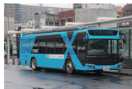
Fig. 3 JTEKT Test Vehicle Used in Field Tests of Autonomous Driving and Bus Stop Precise Arrival
