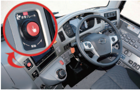
Fig. 13 Hino S'elega Featuring Emergency Driving Stop System (EDSS) as Standard Equipment
