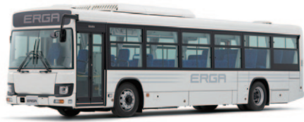
Fig. 15 Isuzu Front Door Erga Bus Changed to a Non-Step Base
