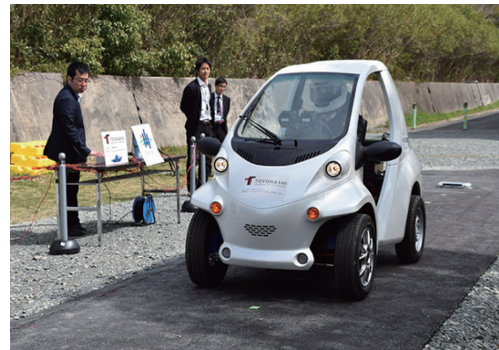
Fig. 7 Road Test of Battery-less EV Using a Tire-based Electric Power Collection Method (42)
