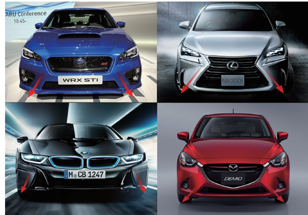
Fig. 5 Example of bumpers with a slanted outward base: Subaru WRX STI (top left), BMW i8 (bottom left), Lexus NX (top right) and Mazda Demio (bottom right)
