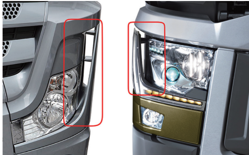
Fig. 3 Example of bumper corner vent adjustments: new Daimler Actros (left) and new Renault T-series (right)
