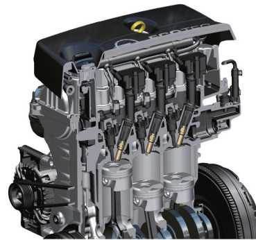
Fig. 21 Direct injection piezo injectors in Opel 1.0-liter SIDI turbocharged engine.
