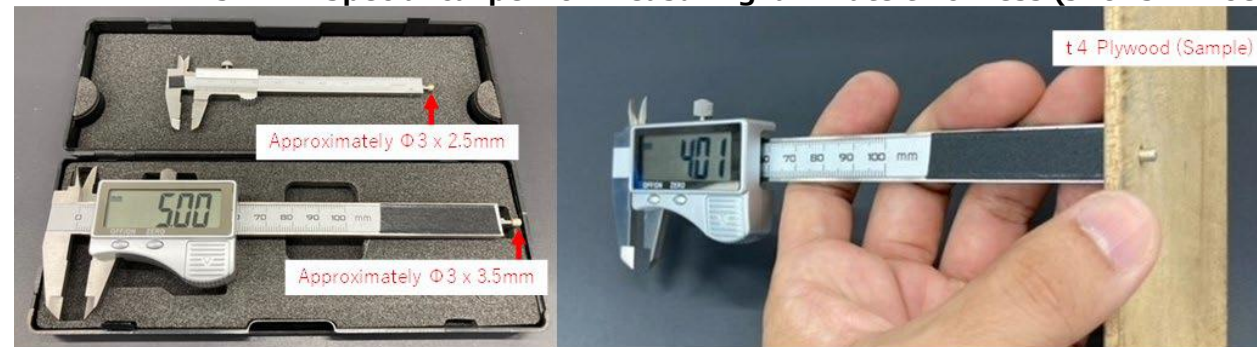
APPENDIX J-IN-1 Special caliper for measuring laminate thickness (J2025-IN-08)
