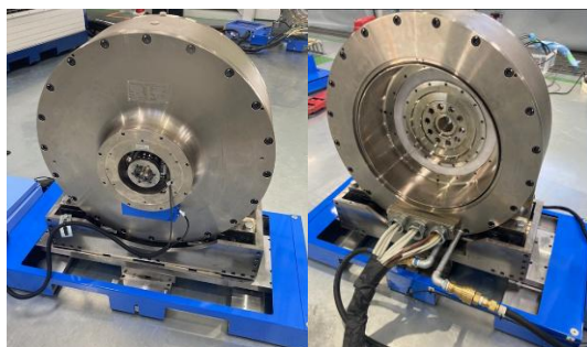
Fig.1 94kW flat-type dynamometer
