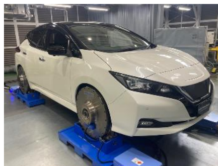
Fig.3 Vehicle equipped with 94kW flat-type dynamometer
